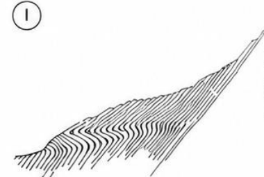
Kink band slumping S-shaped deformation of rock lamellae due to slope creep A. PREH (2004)
