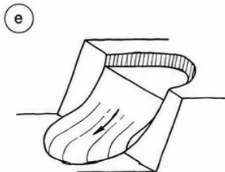
Sliding of a rock block on a single or on two discontinuities Translational sliding R.E. GOODMAN & G.-H. SHI (1985)
